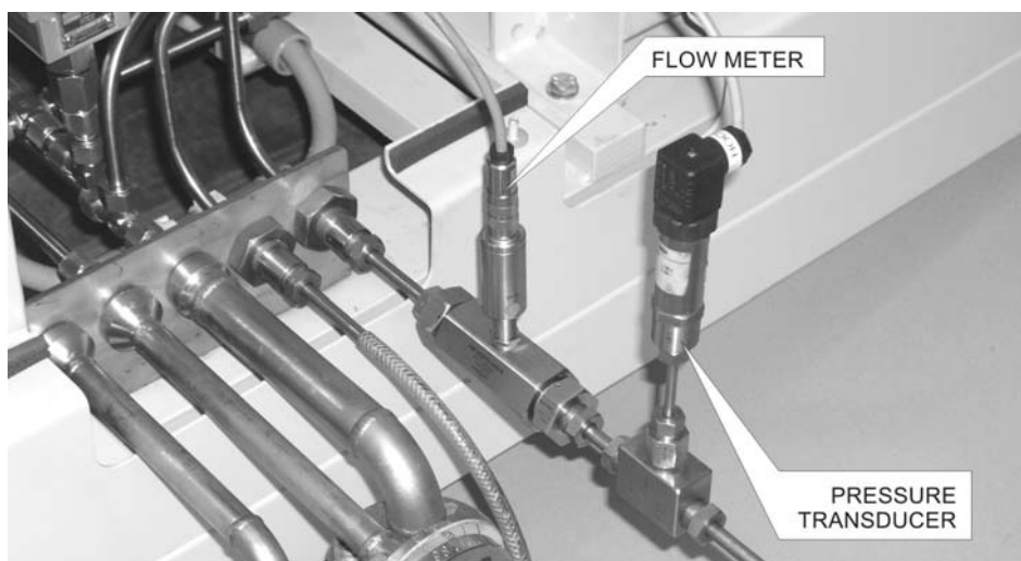
Figure 3: Measurement equipment installed at the discharge side of the pump
